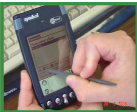
Linen inventory coming in and going out of a laundry services facility (like Eggleston) can be recorded into the LinenWeb® system remotely via a small handheld device (or PDA).
